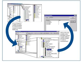
**Figure 3.** DeltaV Console.CONNECT for Bailey configuration includes easy configuration with predefined templates available.
