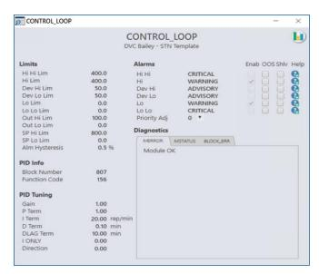
**Figure 2:** Station (STN) block detail display gives access to PID tuning parameters, while maintaining a seamless appearance with other DeltaV standard faceplate and graphics.
