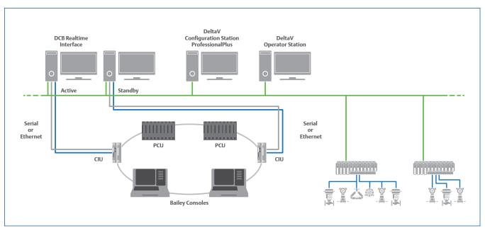
**Figure 1.** Bailey controller information is available in DeltaV workstations for operator interface, events, and history collection, in either simplex or redundant configuration of the DeltaV Console.CONNECT for Bailey interface.
