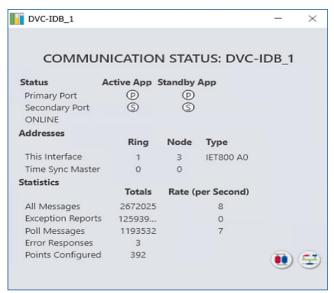
**Figure 5.** Called from a toolbar button, the communications status faceplate provides detailed information about the health and performance of the interface.
