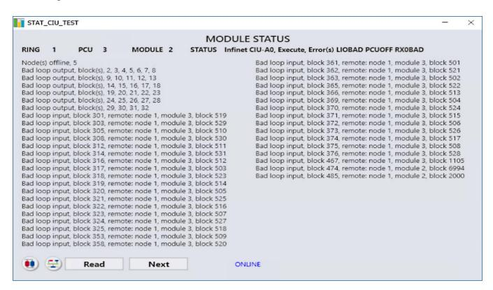
**Figure 6.** Called from a toolbar button, the module status faceplate provides information about the individual blocks inside the Bailey controllers for easy internal block troubleshooting.
