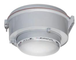
Appleton Mercmaster LED Low Profile Series Luminaires have a compact, lightweight, low-profile design suited for low mounting heights. Six standard mounting hood designs allow for mounting in any location and four different globe options, clear and diffused polycarbonate, clear glass, or prismatic glass refractor, enable customization to the application requirements.
