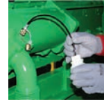
Figure 9: Sampling a Jenbacher gas engine with a needle probe valve (Ref : GE)
