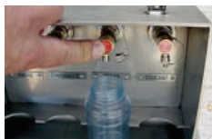
Figure 5 and 6: Fluid Sampling station for mining equipment (Ref: Fluid transfer Systems Welshpool Australia)
