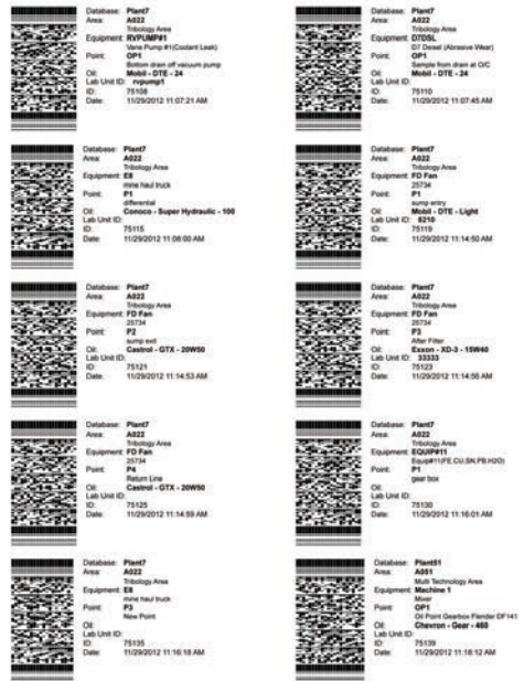
Figure 12-5: A “route” of points represented by sequenced machine readable sample labels – generated from Emerson OilView
