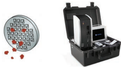
Figure 3: Pore blockage particle counter used in the Q5800 Expeditionary Fluid Analysis System
