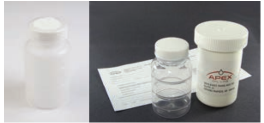
Figure 15: Opaque (HDPE) and clear (PETE) 120 ml sampling bottles (ref: Apex oil lab )
