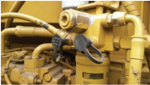
Figure 1: Sampling points preinstalled on a CAT 320D excavator. Caterpillar SOS program relies on good oil analysis sampling to ensure warranty programs are effective. (ref: Spofford Construction)
