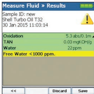
Figure 9: The warning message to the user that free water may be present in a sample up to 1000 ppm.
