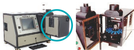
Figure 10: Robotics in SpectrOil M/R spectrometer
