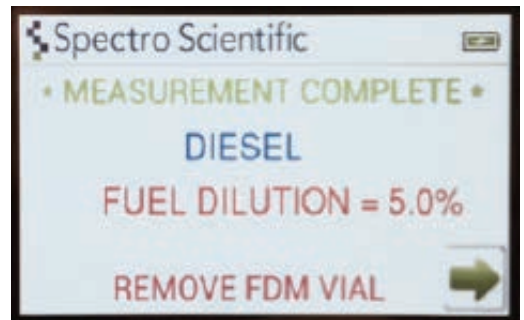
Figure 4: Results screen on the Q6000 FDM showing the % fuel dilution found for a sample using a diesel calibration program.
