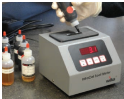
Figure 3: InfraCal soot meter from Spectro Scientific. The sample is simply squirted onto the top glass plate and a determination of soot appears in seconds on the display screen.
