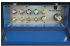
Figure 5 and 6: Fluid Sampling station for mining equipment (Ref: Fluid transfer Systems Welshpool Australia)
