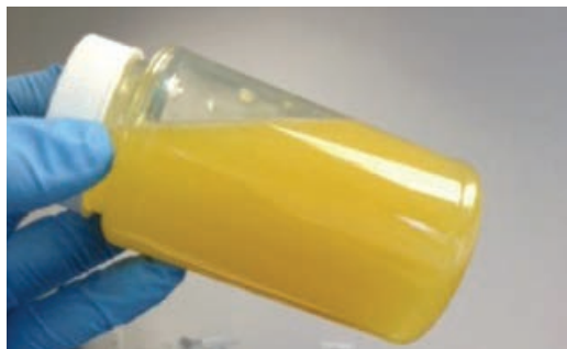
Figure 7: Sample which was shaken vigorously by hand for 30 seconds. To the eye, the opacity looks similar to the homogenized samples even though the water is not uniformly dispersed in the sample.
