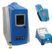
Figure 1-3: Example of on-site oil analysis system for engine test labs including elemental OES, IR spectrometer and fuel dilution meter. The system does not require sample preparation, or chemicals for cleaning. In addition, only 3 ml of oil is consumed for all three tests.
