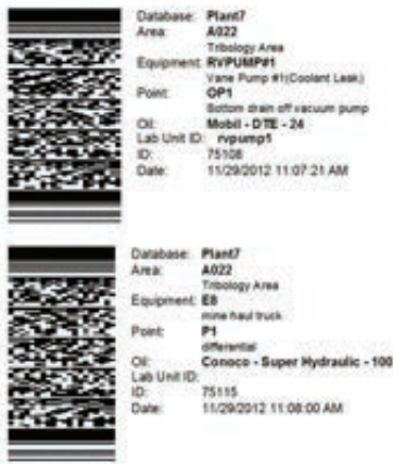
Figure 18: Oil sample bottle labels preprinted with OilView software (Ref: Emerson Process Management)
