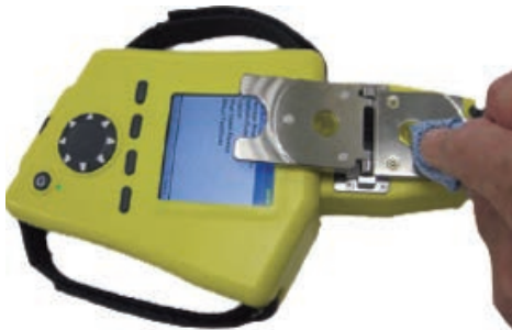
Figure 7-2: Patented flip top cell eliminates the need for solvents to clean
