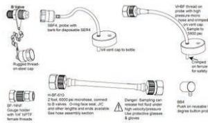
Figure 7: Options available for sampling pressurized valves (Ref: Checkfluid)
