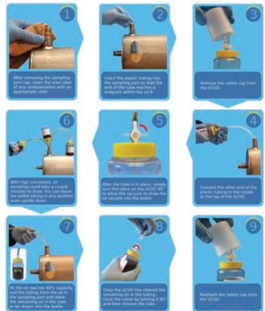
Figure 16: Sampling process using UCVD bottles (Ref: Mecoil)
