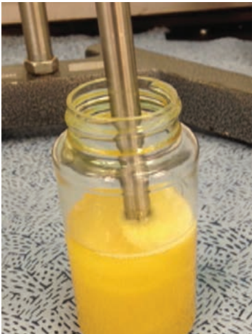
Figure 4: Homogenizing a sample of water-contaminated oil.
