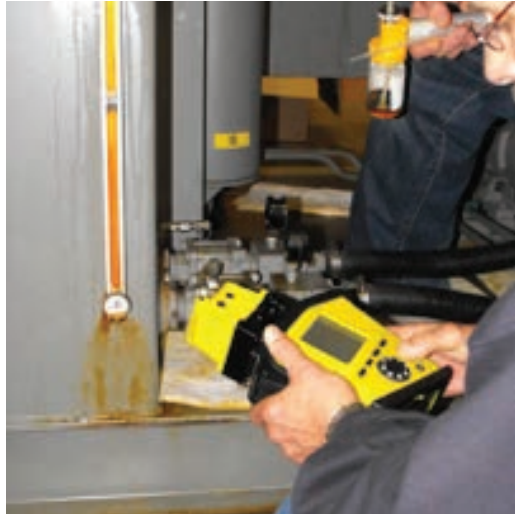
Figure 19: Operators sampling and testing oil condition of a hydraulic reservoir (Ref: Spectro scientific)
