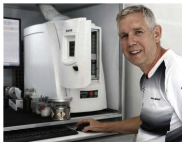
Figure 9: McLaren and Mobil 1 use the SpectrOil 100 Series on the global F1 circuit (Ref: McLaren)
