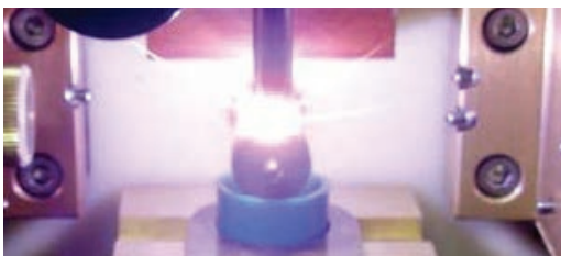
Figure 3: RDE spectrometer sample stand showing oil sample being “burned”
